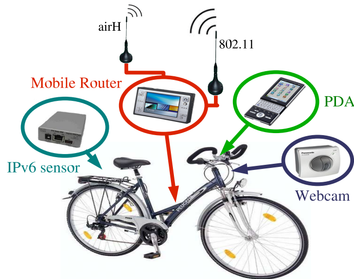
Figure B.2: E-bike. Thanks to the Mobile Router, all devices such as the sensors, the PDA or the webcam can access the Internet and be reached from the Internet, without disruptions.
